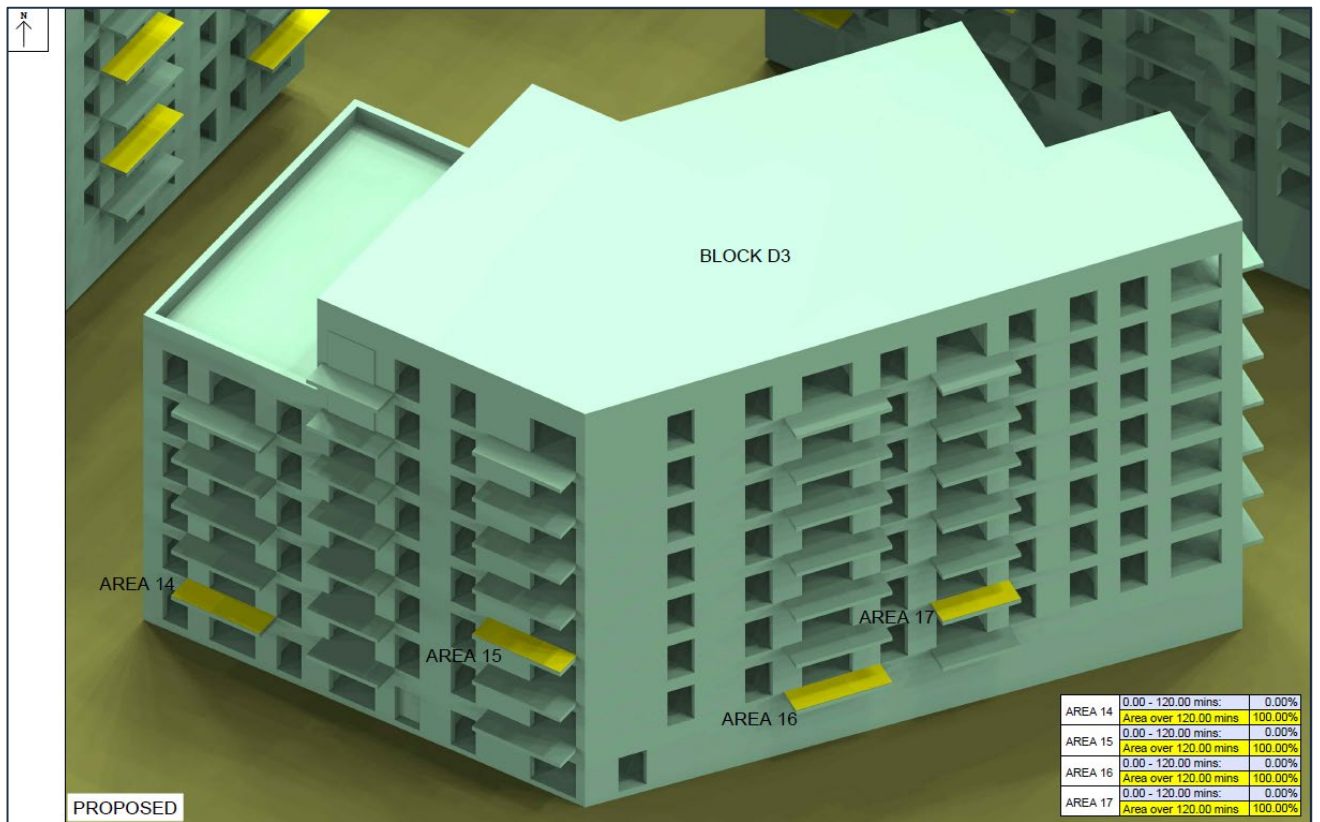
Figure 5 – SHOG Overshadowing assessment for a selection of proposed balconies serving Block D3 (full results located in Appendix III, see drawings BRE/13-20)
